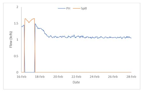
Figure 16. Hourly Flows PWR vs. Spill (Big Cliff Dam)
